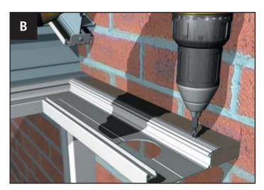
Secure lower section using fixings provided (CRN007)
