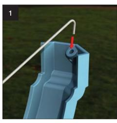
1. Prior to fitting the corner insert the special longer wire tie CRN012, into the corner as indicated
