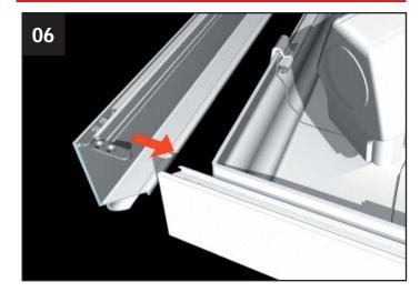
Fit cleats as shown in step 3. Offer up the next middle Cornice section. Continue to support lower section as shown in step 5.
