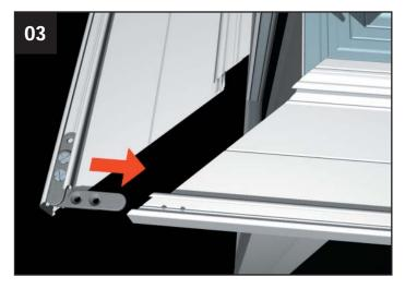
Fit the cleats (CRN001) to the desired side using the fixings provided (CRN006) as shown and assemble the remaining lower sections
