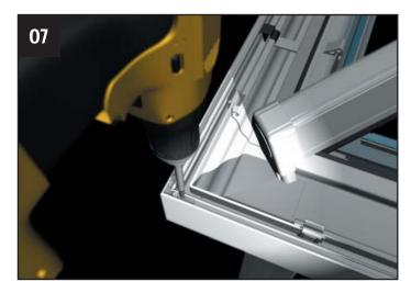
As shown in step 5 it may be advisable to temporarily support the Cornice whilst fixing. Secure corners using the cleats (CRN001) and fixings provided (CRN006).
