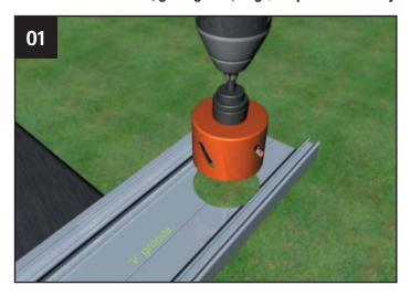
Decide the position of the gutter outlet by lining the extrusion 'v' groove up with the centre of the hole for the down pipe. Using a 73mm dia hole saw, cut the hole for the down pipe in the lower section.
