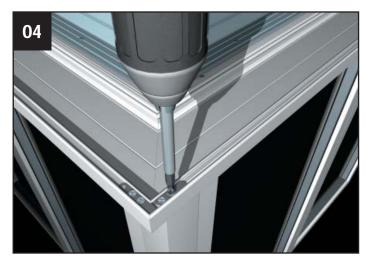
Secure each corner using the cleats (CRN001) and fixings provided (CRN006).
