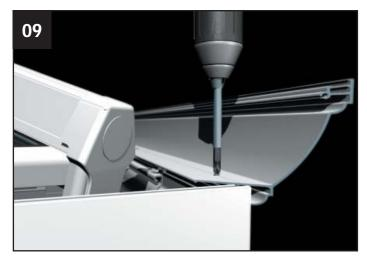
Temporarily support and fit the upper Cornice section, using the fixings provided (CRN007). Secure the corners using the cleat (CRN001) and fixings (CRN006) as shown in step 3.
